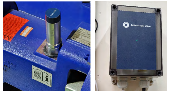
Figure 5. BKV Collect wireless sensor is shown on the left (the QR code, not visible, is on the back of the sensor). The BKV Connect gateway is shown on the right.
